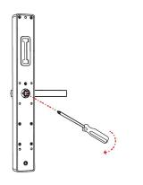
1、Turn the handle on back panel Loosen the inner hexagon screw of the handle counterclockwise
