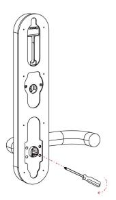
1. Turn the handle on back panel Loosen the inner hexagon screw of the handle counterclockwise
